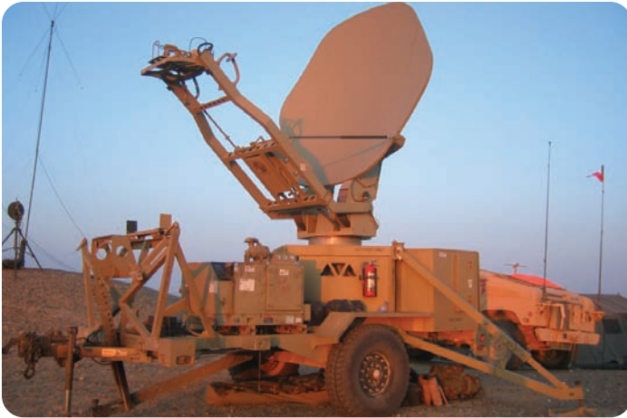
The heart of the JNN program: DataPath's trailer-mounted STT, shown here deployed in Iraq, goes anywhere a HMMWV can.
